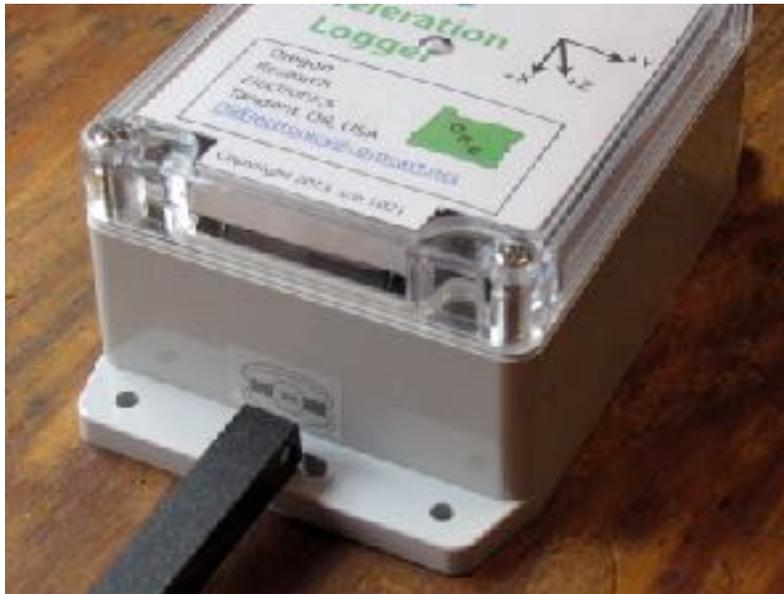
Figure 6-1 Start/Stop Switch Activation
