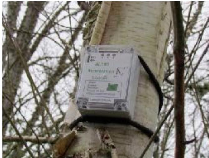
Figure 6-9 Bungee-Secured Accelerometer
