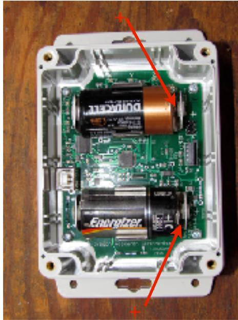
Figure 6-4 Battery Orientation
