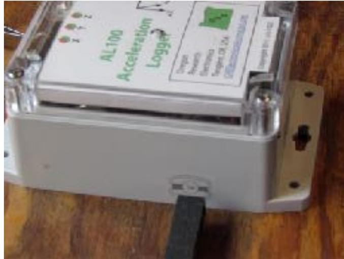
Figure 7-1 Activating Test Mode
