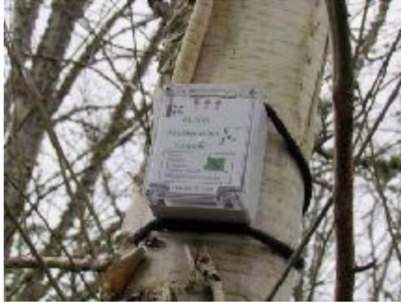
Figure 1-7 Logger Mounted in Tree Using Bungee Cord
