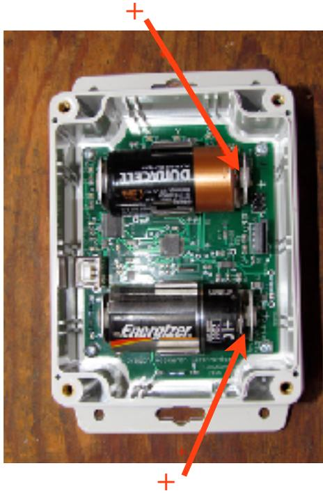
Figure 1-3 Battery Orientation
