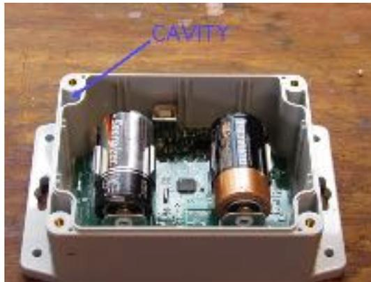
Figure 6-8 Water Retaining Cavities
