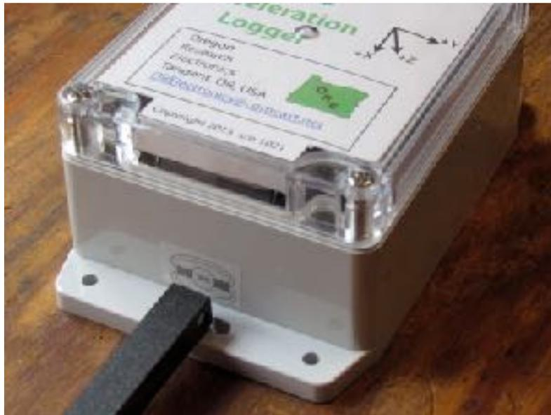
Figure 1-5 Using Wand to Start Recording
