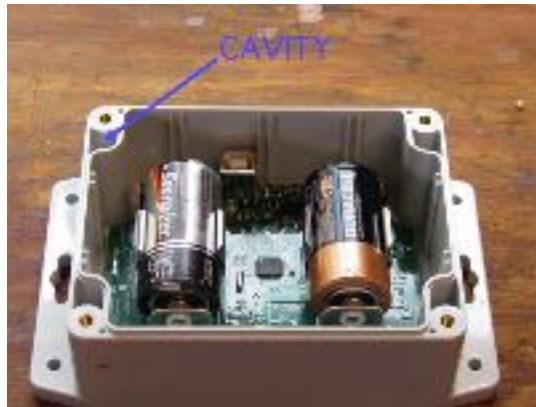
Figure 6-8 Water Retaining Cavities
